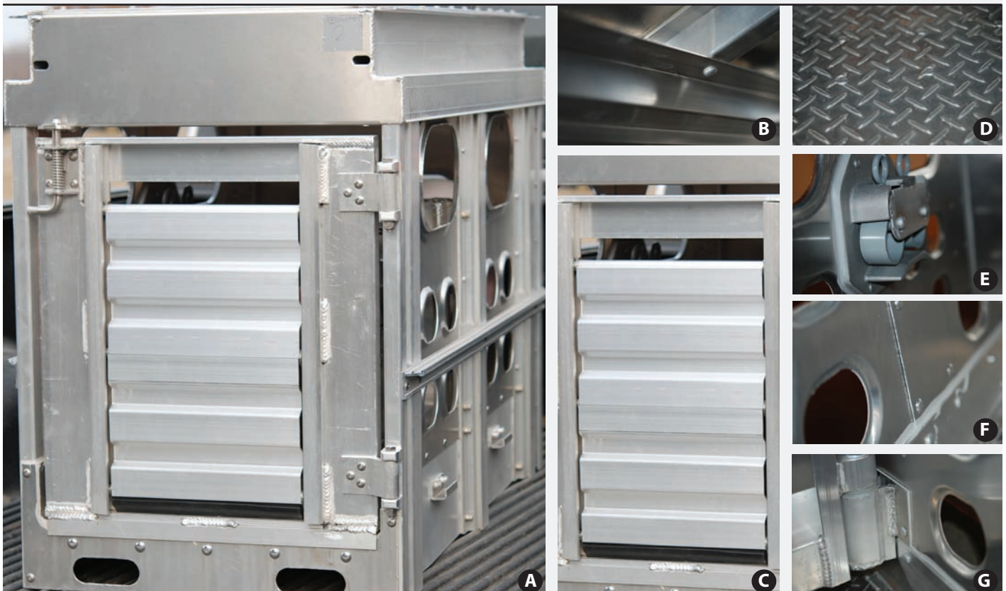
Figure 1: A: 1:61 scale model of a full-sized standard livestock trailer used in the transportation of commercial swine; B: Models were composed of aluminum smooth-sheet side walls welded and riveted to tubular extruded aluminum cross-members; C: Hinged aluminum simulated roll-up rear door; D: Aluminum alloy diamond-plate flooring; E: Latch; F: Overlapped seam at the side post; and G: Center divide gate. Dimensions were 0.62 m width × 0.82 m height × 1.11 m length.
