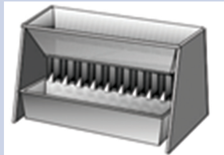
Figure 6: Quartering method. Reproduced with permission from Herrman. 3
